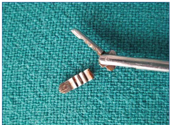
[Table/Fig-2]: Broken prong after retrieval.
